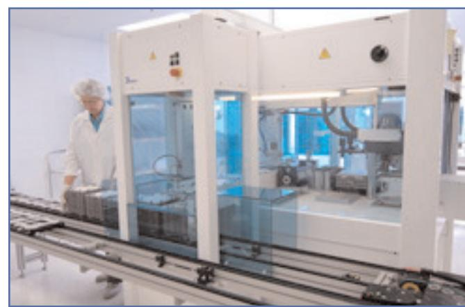
Baccini automated printer and collator system with layer to layer accuracy of ± 0.0005"
